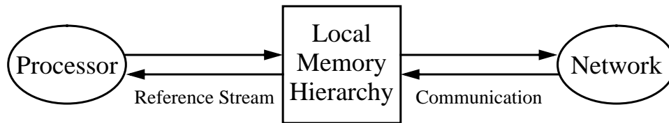
Figure 7.1: The local memory hierarchy in a DSM sits between the processor and the network.
