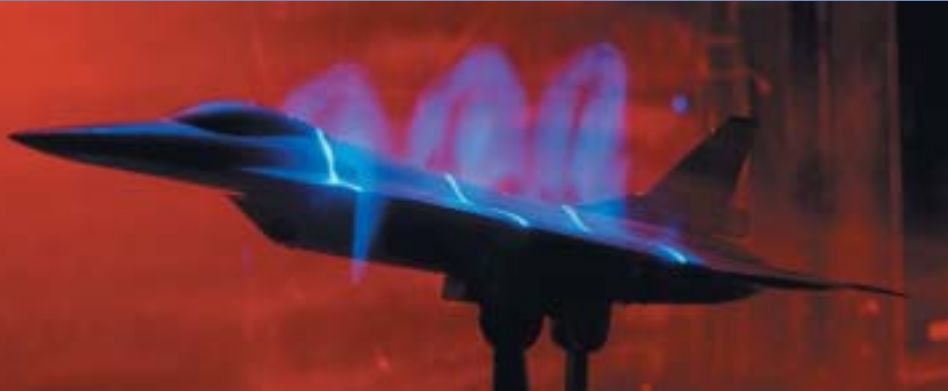
F-16XL Scamp Flow Visualization Test at NASA's Langley Research Center
